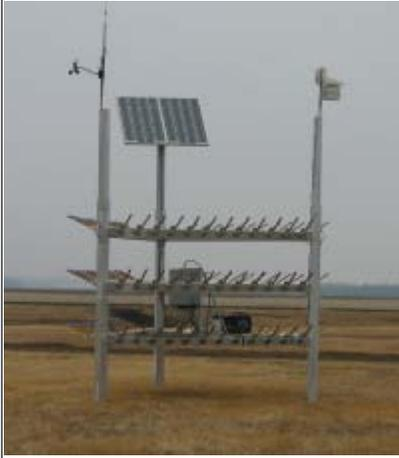
WMI offers the latest in ground-based pyrotechnic applications, specifically, the ground-based flare tree, or GBFT. Our GBFT incorporates a “tripod base”, which provides exceptional stability in even the most extreme weather conditions, and easy leveling.
