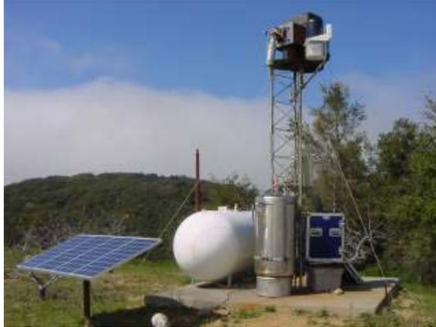
WMI has designed state of the art ground based silver iodide generators for seeding orographic clouds. The generators burn a mixture of acetone and silver iodide that produce a silver iodide plume which is ingested by the cloud.
