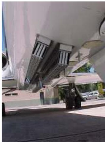
WMI racks for ejectable flares are mounted on the belly of the aircraft fuselage. Each rack holds 102 cartridges. When fired, the pyrotechnic is ignited and ejected from the aircraft. In this configuration, the WMI Lear 35A is equipped with four 102-count racks for ejectable glaciogenic pyrotechnics, a total of 408 flares. [Click to enlarge image.](#)
